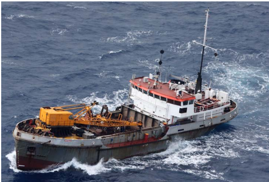
Above seen the 1969 built hopper grab dredger KMC PELLICAN under tow of the 1981 built COMARCO OSPREY offshore Malta on Wednesday 6th April, 2011 heading to Suez Canal. Photo : Cpt. Lawrence Dalli - www.maltashipphotos.com ©
